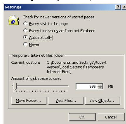
3. Ensure that the **Automatically** radio button is enabled, and click the **OK** button.
